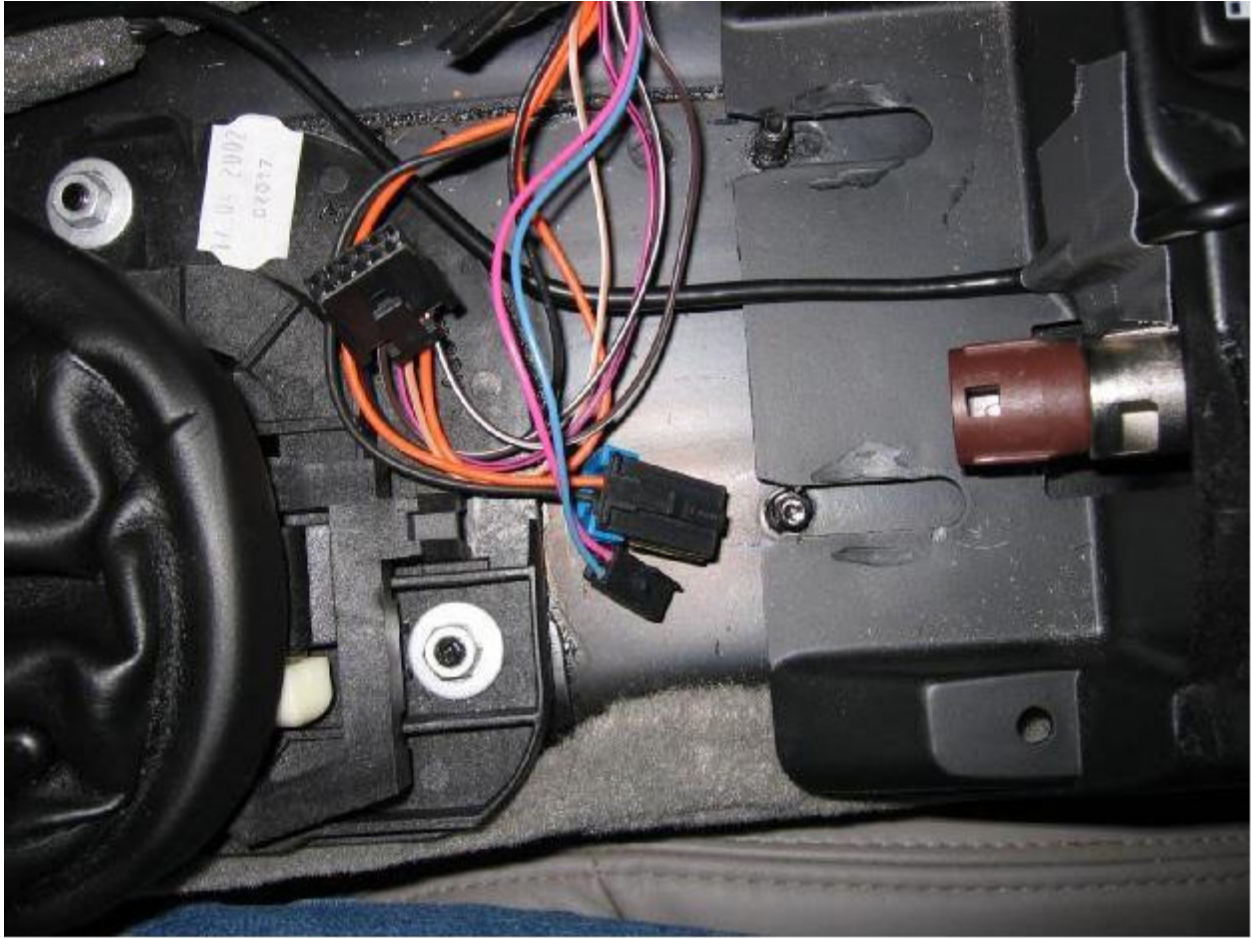
Route the black iPod cable into the center console storage area as shown above.
